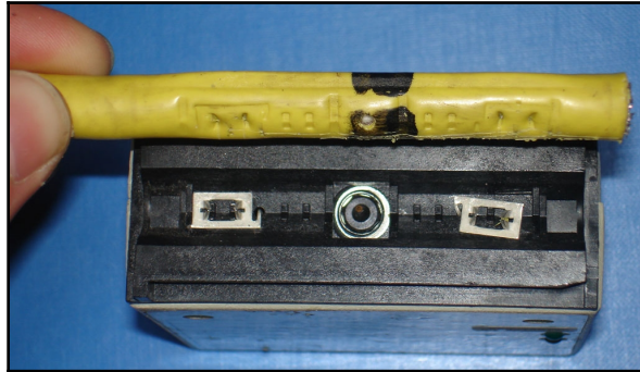
Figure 8.3: Vampire tap showing bite marks
