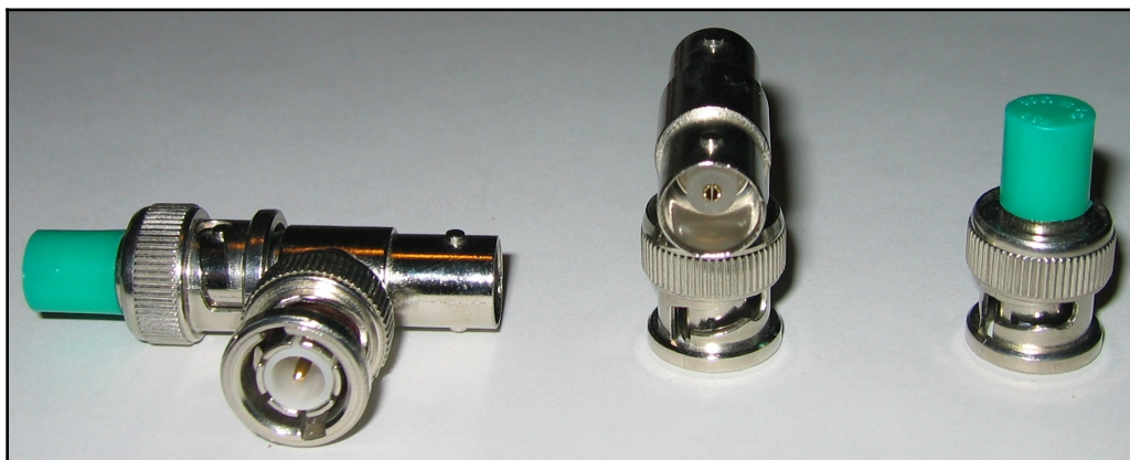
Figure 8.6: T-piece connectors left and center, and [green] terminators
